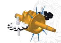
Radial loads act on both the top and bottom of the main rotor
