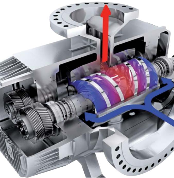
L4 Pumps are selfpriming screw pumps with two screws in double volute and hydraulically balanced design. The drive torque is transmitted from the double helix drive screw to the likewise double helix idler screw via herringbone gears.
