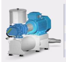
**Footprint** · with noise enclosure: 770 x 1,630 mm without noise enclosure: 700 x 1,574 mm Total height: 1,290 mm Blower inside: 1 x RBS 55 Motor rated power: 22 or 30 kW Piping connection: DN65 (1 outlet)
