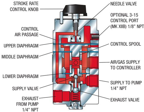
The MK XIIA Controller operates on the same operating principal as the MK X Controller. The MK XIIA has the same upper and lower chambers, but are separated with flexible diaphragms rather than sliding seals. A capillary tube, controlled by a needle valve, transfers the air/gas supply to the pump from the lower to the upper chamber.
