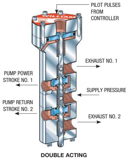
The PNEUMATIC RELAY is a pilot-operated valve designed to provide the higher air or gas flow rates necessary for for higher pressures from 100 to 150 psi. The PNEUMATIC RELAY is actuated by the pulses produced by the OSCILLAMATIC® CONTROLLER.
